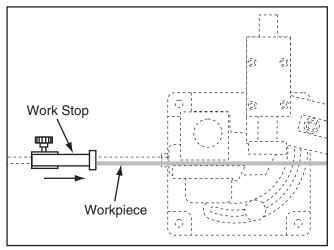
Figure 16. Using work stop.
